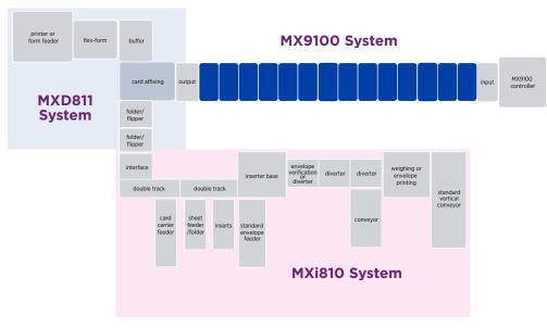
Note: The folder/flipper capability is only available with the High-Speed Folding Kit.
